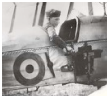
An observer of the Royal Flying Corps in a BE2c reconnaissance aircraft demonstrating a C-type aerial reconnaissance camera fixed to the side of the fuselage
